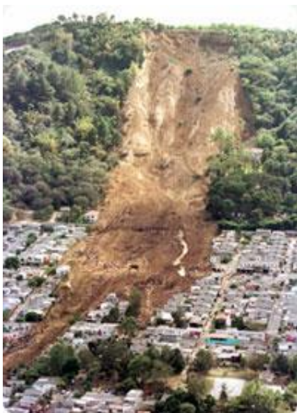
This landslide in El Salvador destroyed many homes in the valley below the hill. It happened after recent logging on the hill.
